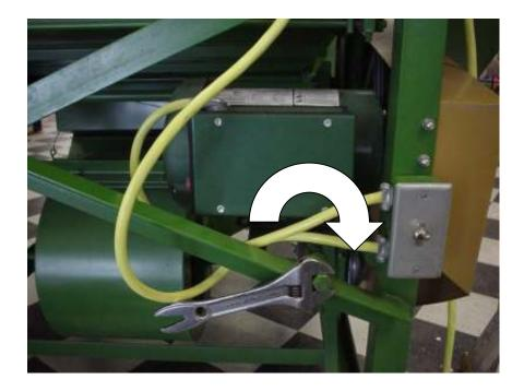
TO SLOW MACHINE DOWN TURN MOTOR MOUNT BOLT CLOCKWISE SO THAT IT TIGHTENS THE BELT CAUSING THE ADJUSTABLE PULLY TO SPREAD MAKING THE PULLY SMALLER. TO SPEED MACHINE UP TURN BOLT COUNTER CLOCKWISE TO LOOSEN THE BELT CAUSING THE PULLY TO COMPRESS MAKING IT BIGGER.
